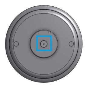
60. Next, create a new gear, called Motor Gear, at this point, using the Spur Gear Feature:
